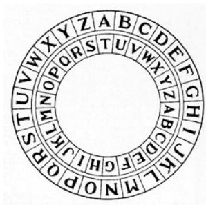
FIG. 1: Representation of the shift cipher as two concentric rings: the outer is the plaintext and the inner, the corresponding ciphertext. For an alphabet with N characters, there are N - 1 implementations of this cipher.
